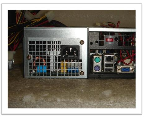
2. There are two sets of screw & nuts in the accessory box. Using them to secure the rear bracket.
